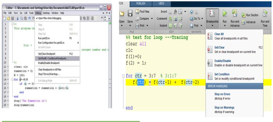
We can use the Matlab debugging tool Set/Modify Conditional Breakpoint to check the execution of the program when n=0.
